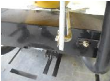
C) Fix the adjusting bar on the proper hole of the lever and shutter by 2 WASHER M10 and 2 RPIN
