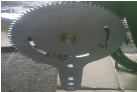
I) Assemble the Lock nut M10 and tighten
