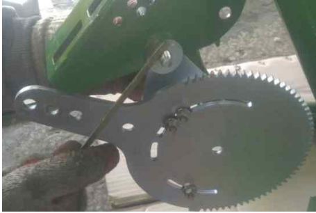
E) Paint the grease on Washer
