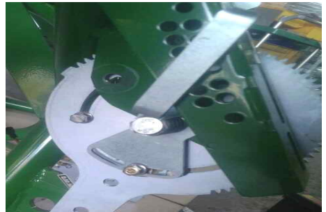
H) Assemble the washer M10
