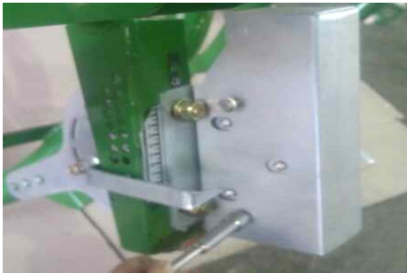
Y) Tighten DC motor cover
