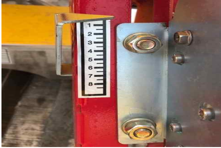
X) Set gage pin on gage level and tighten(Closing)
